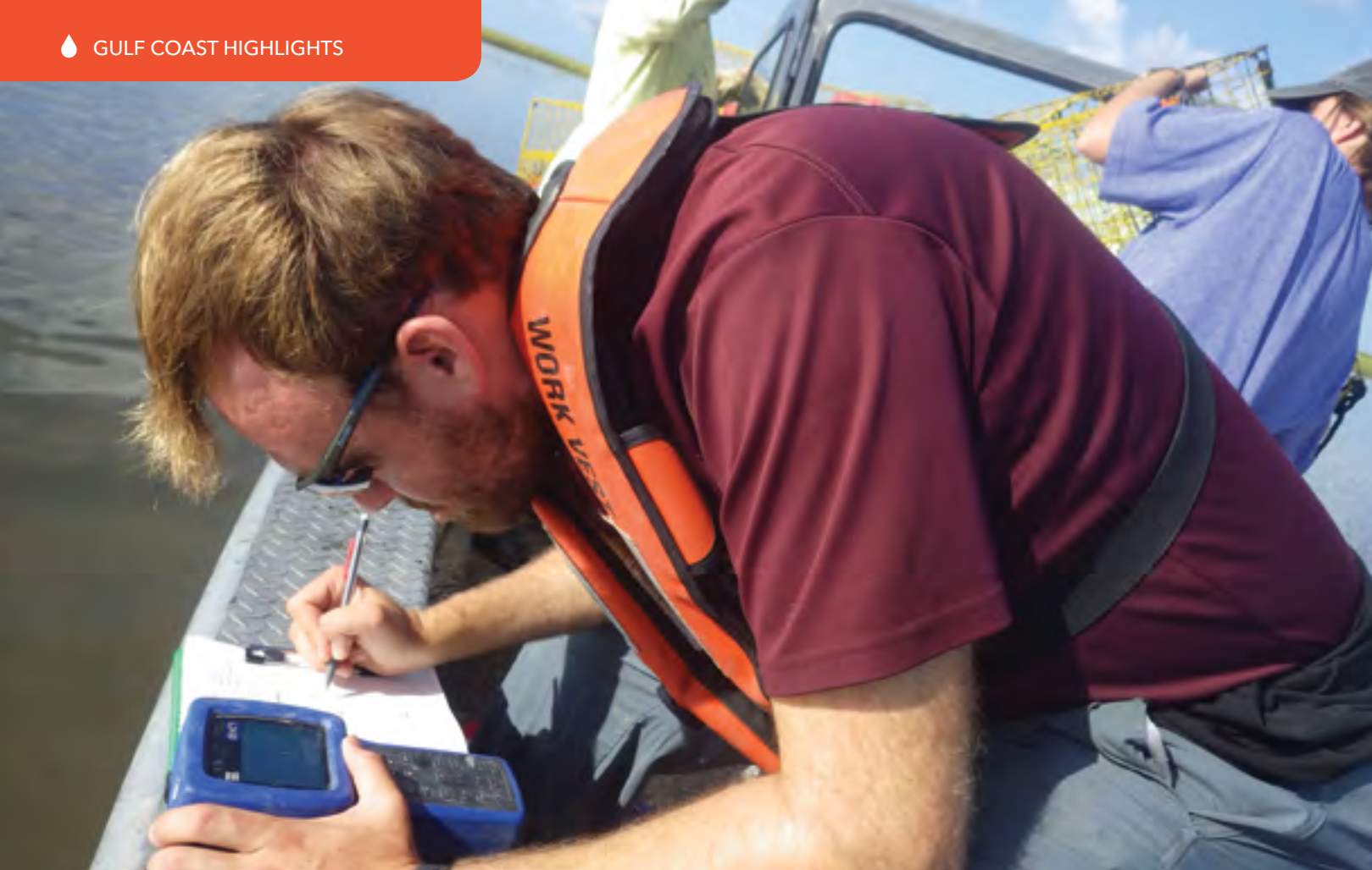
Above: Leland Moss, research associate, records data for NOAA from a YSI EXO multiparameter sonde handheld.
