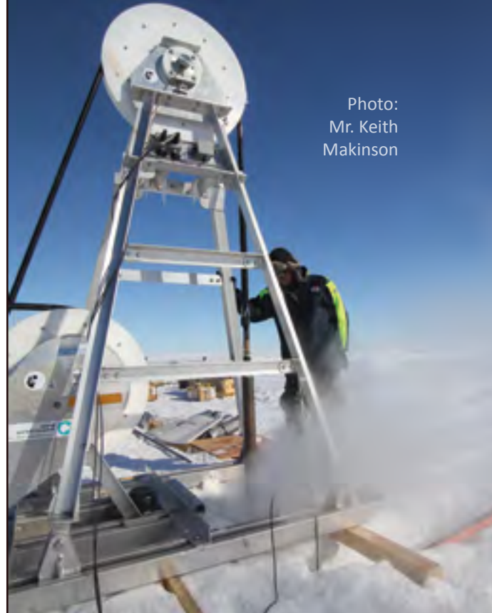
The challenging task of ice drilling to make way for these SeaGuard instruments.
