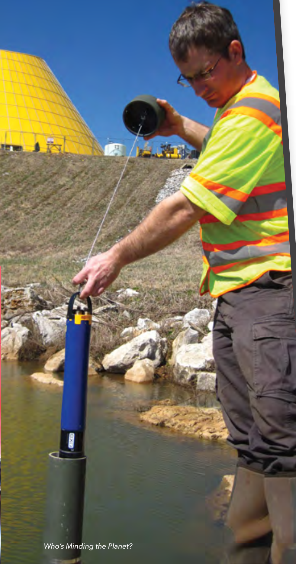
A geologist uses an EXO sonde to monitor changes in water quality in a sinkhole adjacent to the Corvette Museum. Photo: Dr. Jason Polk
