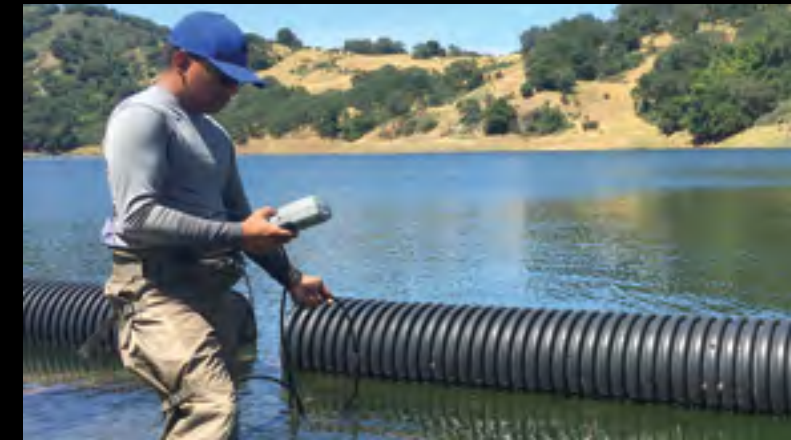
Norm Ponferrada monitoring water quality using a YSI Model 556 at Guadalupe Reservoir in California. Photo: Norm Ponferrada
