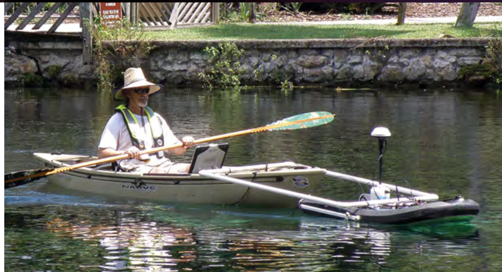
Mitch Wainwright of the St. John River Water Management District (SJRWMD) figures he paddled more than 200 to 300 miles while measuring depth, flow and velocity of a six-mile reach of the Silver River in 2015 and 2016.
