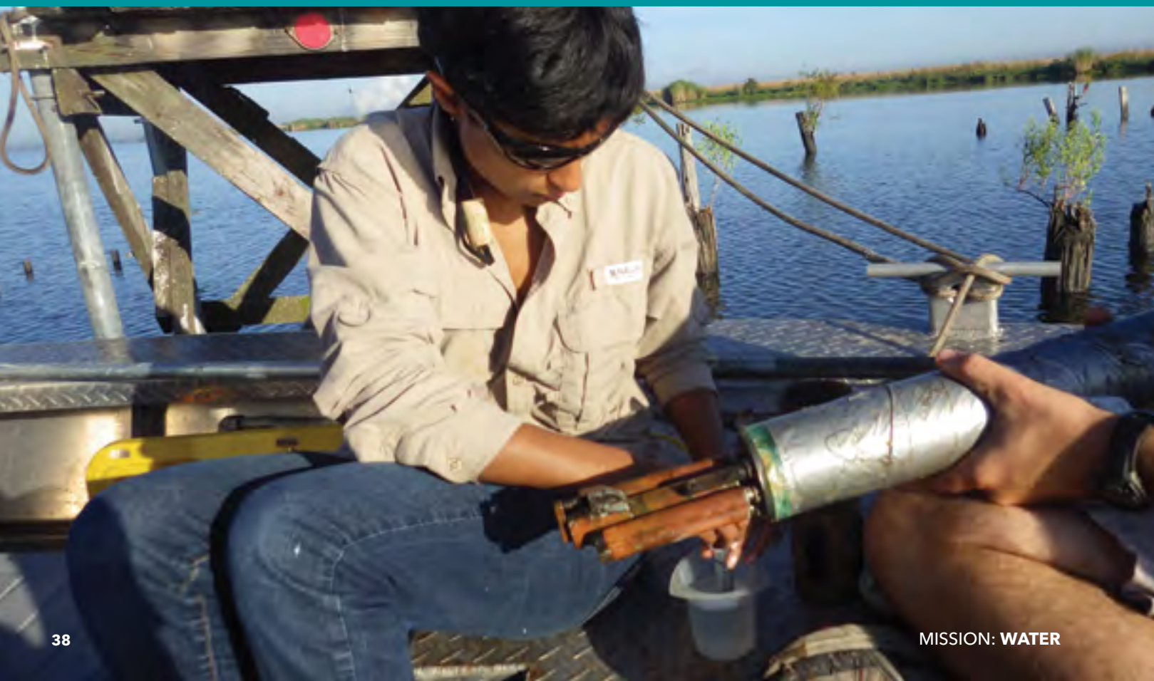
Above: Leland Moss, research associate, records data for NOAA from a YSI EXO multiparameter sonde handheld.
